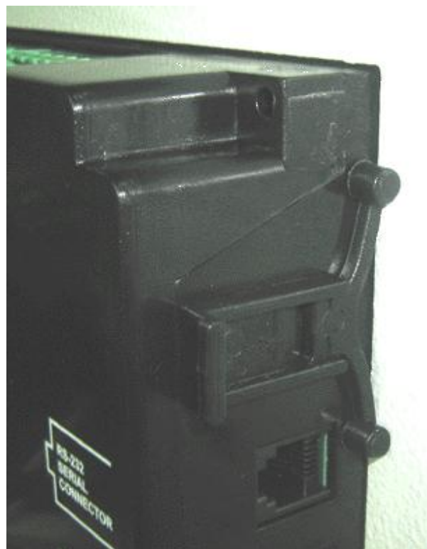
Installation of self retaining type bracket
